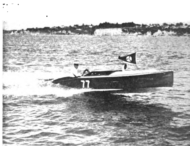
Fleetwing at Speed. Judging by the Illustrations It Seems That She Would Run on a More Even Keel If Her Motor Was Moved a Few Inches Further Forward
